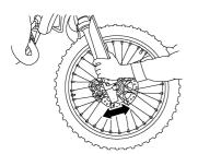
FAU23283 Checking the wheel bearings
